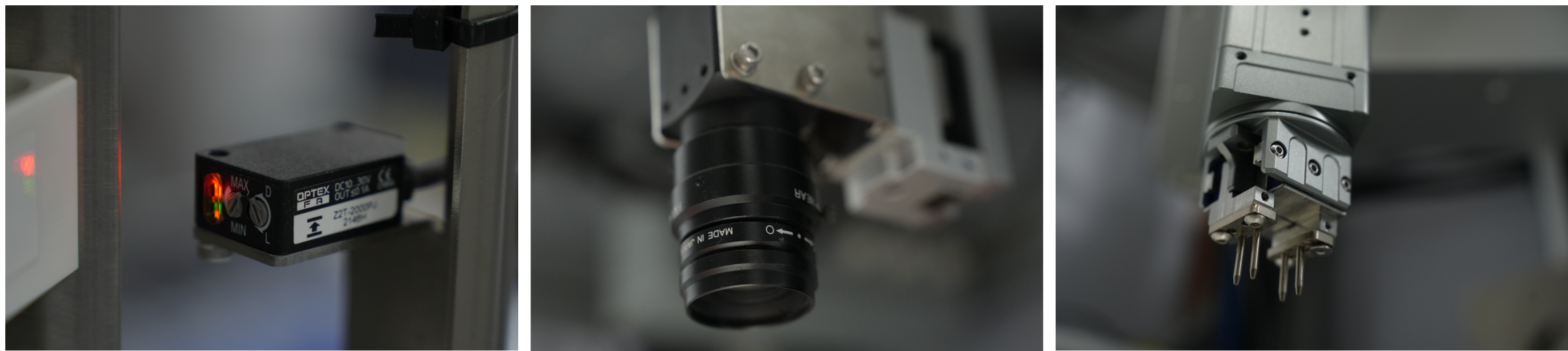
Figure 1. The equipment used in the system, from left to right, are infrared transceiver sensor, smart camera, and claw.
